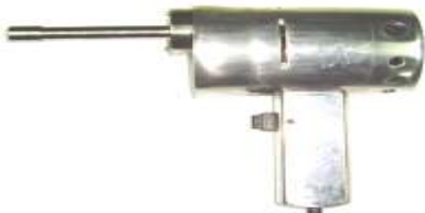
Electric Oscillating Plaster Cutting Saw- Metal Body
